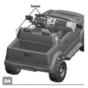
Insert two screws through the back of the seat and into the vehicle.
